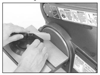
Figure 18. Disc sanding with a miter gauge.
